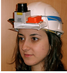
Figure 1: The test person with Hokuyo URG laser scanner and XSens IMU mounted onto her helmet.
