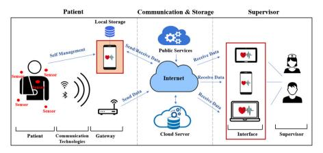
Fig. 1 A typical architecture for a remote health monitoring system (The red boxes show the role of apps in remote monitoring process. The shaded box shows the scope of HealMA) (Color figure online)
