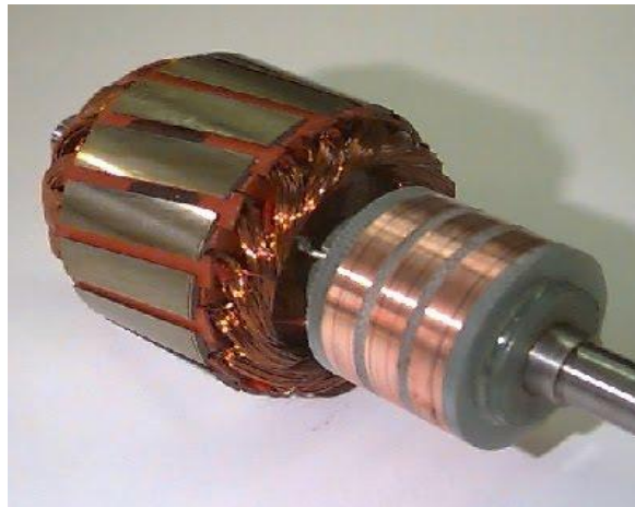
Fig.3: Construction of Slip ring rotor
