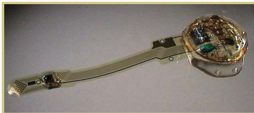
Figure 2. Retinal stimulator for the Healthy Aims retinal implant system. The electrode array is 4 × 5.5 mm, and the electronics is approximately 25 mm in diameter.
