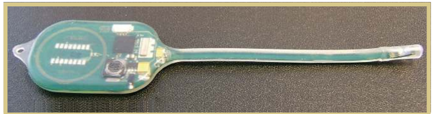
Figure 6. Fully implantable wireless sensor for the intracranial pressure monitoring system.
