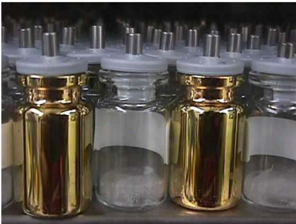
Figure 1. Arrangement of gold-coated vials and clear vials on the freeze dryer shelf. Note the steel tubes inserted into the stoppers.
