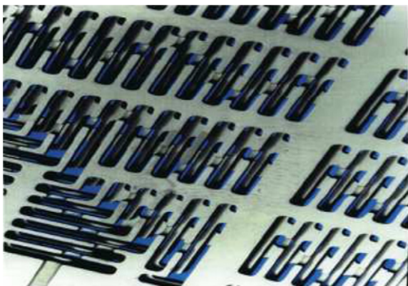
Fig. 17. Layers of slotted plates forming flow paths [51].
