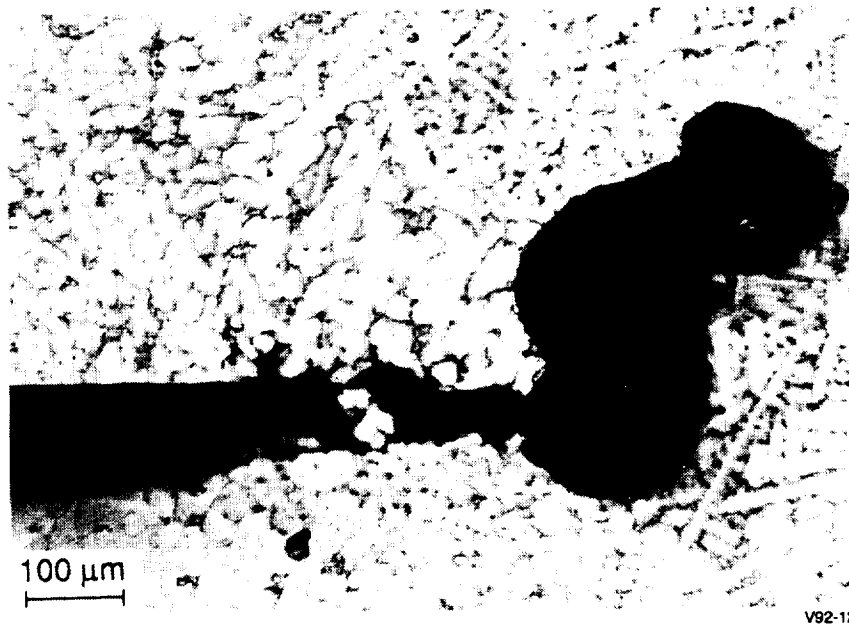
Figure 24. Optical Micrograph of a Pit in Condenser End Cap Crevice
