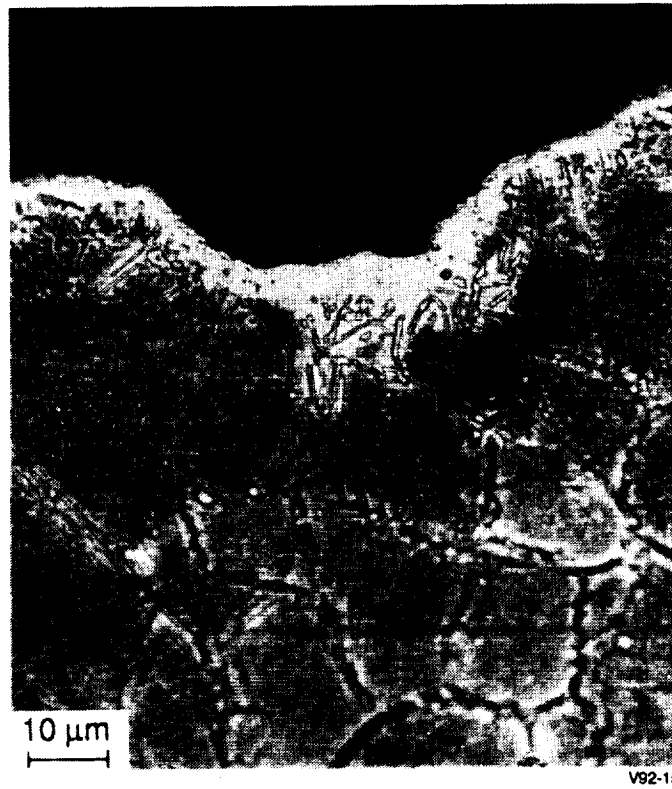
Figure 18. Optical Micrograph of Inconel 718 Surface Layer (White) in Condenser
