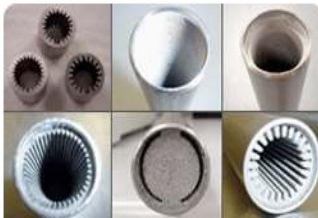
Figure 5. Various wicks structures (clockwise-axial grooves, mesh screen, sintered metal powders, sintered metal powder grooves (fine grooves), sintered slabs, sintered metal powder grooves).
