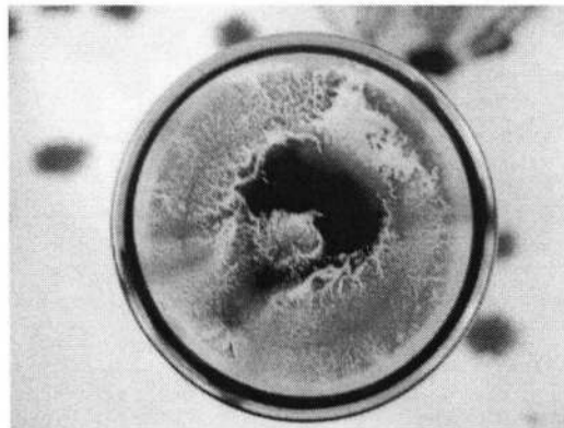
Fig 5.6.3 Example of nanoparticles aggregation after 4 weeks of settling.
