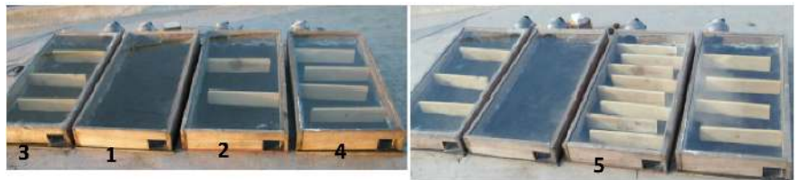
Figure 5. Collector models with installed baffles: Model-1: ordinary collector, Model-2: collector with 2 baffles, Model-3: collector with 3 baffles, Model-4: collector with 4 baffles and Model-5: collector with 8 baffles.
