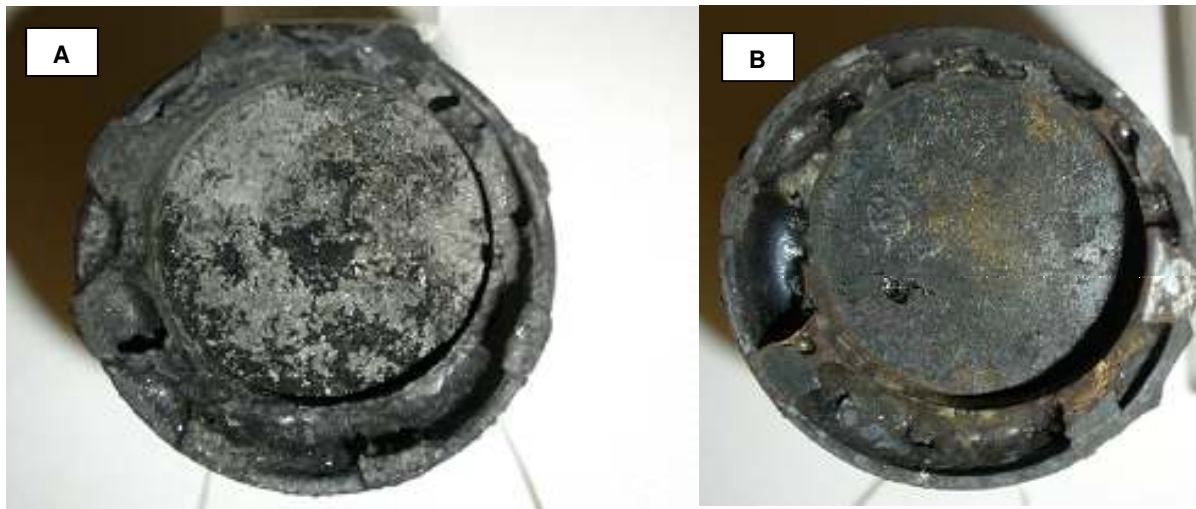
FIGURE 7.2: Top view of the cup containing solidified mould flux (SPH-KA1) with titanium oxide.
