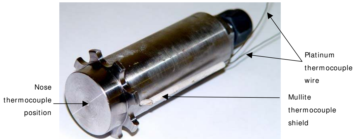
FIGURE 4.8: 310-Stainless steel probe.
