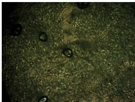
FIGURE 11: POM micrograph of PLA/PBAT (30/70) in the quenching process.
