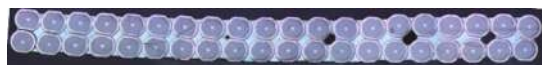
Fig. 3. A cross-section view of the Rutherford-type cable produced at LBNL with B215 strand.
