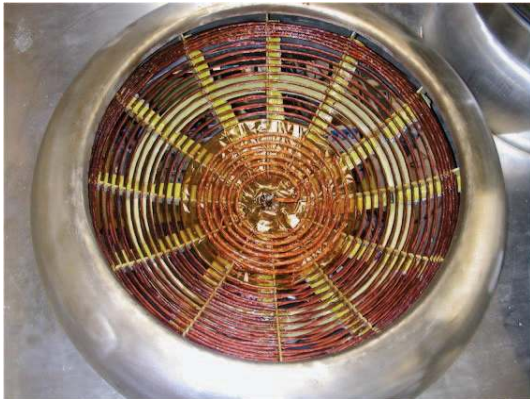
Fig. 12: Induction cooker with variable turn pitch coil
