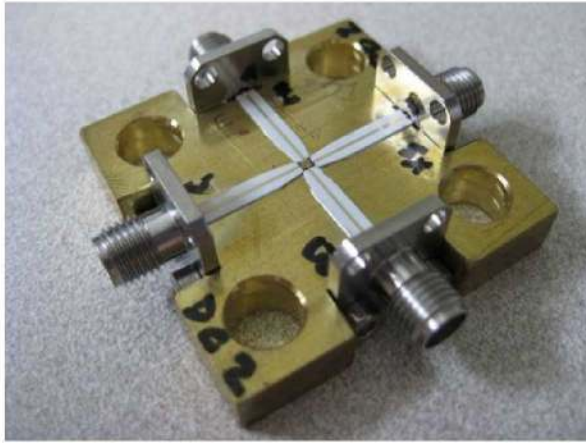
Fig. 2. An example of a high-speed package used for the heavy ion experiments described here and for earlier pulsed laser experiments [12]. This image shows the brass ground plane, the bulkhead 2.9 mm coaxial connectors, microstrip transmission lines, and the DUT tile in the center. The brass substrate is approximately 3.8 cm on a side. The DUT tile in the middle is 1 mm 2 .
