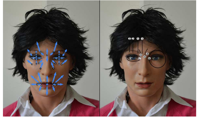
Fig. 2. Mapping between servo motors positions and Action Units of FACS
