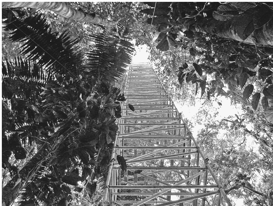
PLATE 1. Mobile aluminum scaffolding tower used for sampling foliage in a tropical rain forest. Photo credit: M. G. Ryan.
