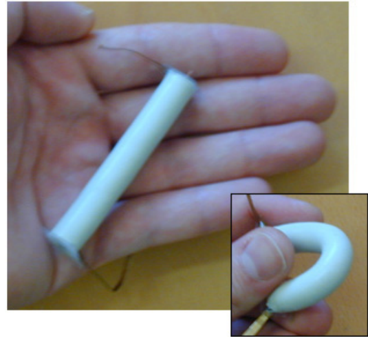
Figure 8. Pictures of a prototype of the new type of dielectric elastomer actuator.
