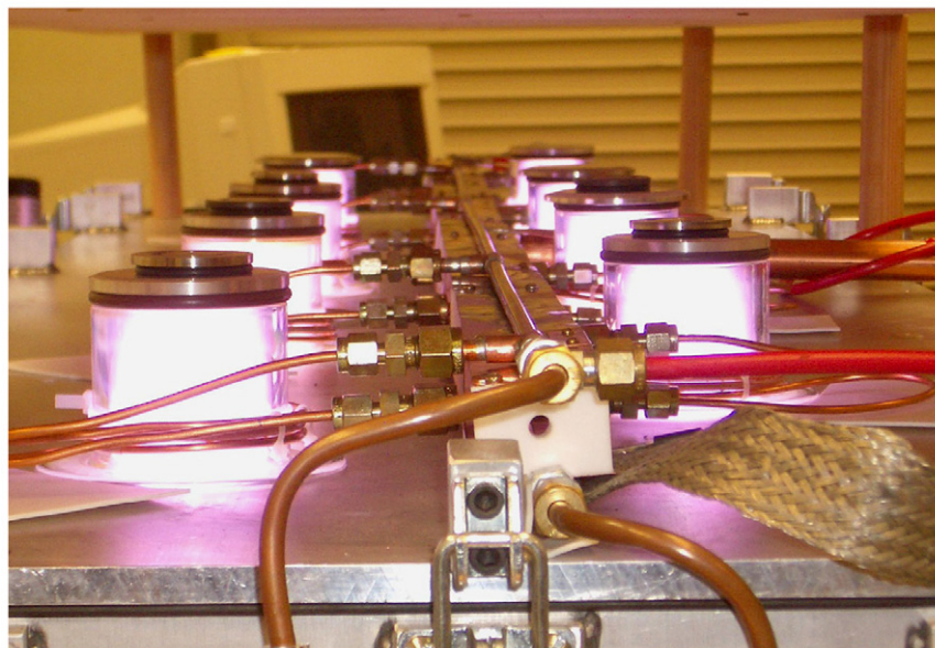
Figure 58. An eight-tube PM helicon array powered from a rectangular 50 \Omega transmission line.
