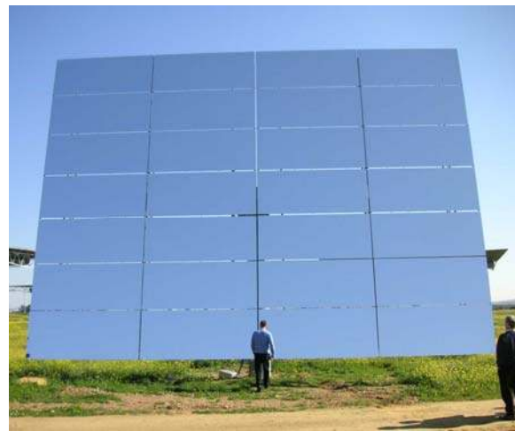
Figure 2-8. Solucar heliostats. A 69\text{-m}^2 model is shown at top. The PS-10 heliostat at bottom measures 121 \text{ m}^2 . Cost of PS-10 heliostat is 140 \text{ Euro/m}^2 .
