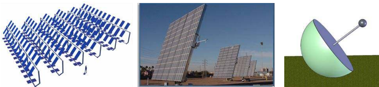
Figure S-5. In the mega-ganged heliostat proposed by DLR (left), up to ~500 m 2 of multiple facets are coupled via a common drive. In the mega-helio proposed by Arizona Public Service (center), an existing 320-m 2 PV tracker would be converted to a heliostat. The water-ballasted heliostat proposed by New Mexico Tech (right) is moved by pumping water between internal chambers. The ball at the end the post is a counterweight.
