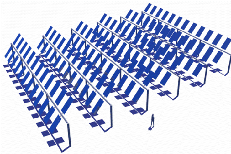
Figure 2-11. In the ganged concept, multiple facets are coupled via a single common elevation drive and single common azimuth drive. Sizes as large as 488 m 2 are believed possible.
