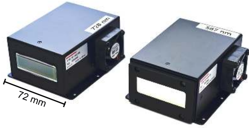
FIG. 10: Two Hamamatsu PMT array modules H11460-20 without (left) and with (right) an attached interference filter. The detector geometry is shown in Figure 11.
