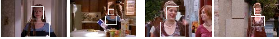
Figure 3: Matching characters across shots using clothing appearance. In the two examples shown the face is difficult to match because of the variation in pose, facial expression and motion blur. The strongly coloured clothing allows correct matches to be established in these cases.
