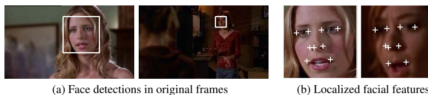
Figure 2: Face detection and facial feature localization. Note the low resolution, non-frontal pose and challenging lighting in the example on the right.
