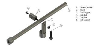
Figure 4. BC3 boccia helmet stick assembly
