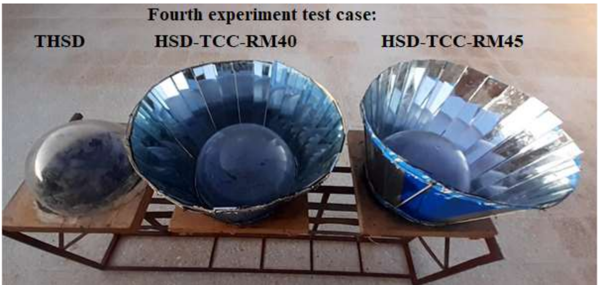
Fig. 3. The pictorial view of the hemispherical solar distillers actual experimental.
