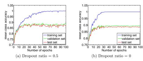
Figure 8: Demonstration of the impact of dropout. It shows that the dropout strategy shall be used cautiously. As seen in (a), the learning process becomes slow and fluctuated on ICPR2014 cell dataset, when dropout is applied. A better learning process is obtained in (b) after removing dropout.
