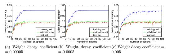
Figure 7: Demonstration of the impact of weight decay. It shows that a smaller weight decay coefficient seems to be a safer choice, while a larger coefficient, e.g., 0.005, could destabilize the learning process.
