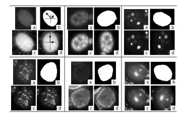
Figure 2: Example cells of six classes in ICPR2014 dataset and their corresponding preprocessed and aligned images. There are four images for each cell: (a) the original image; (b) the mask of this cell image (we do not take advantage of it for training the CNN); (c) the preprocessed image when the original image is applied contrast normalization and resized; (d) the aligned image when the contrast normalized image is aligned by PCA and then resized.
