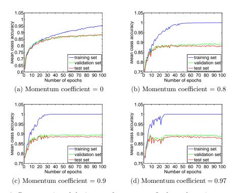
Figure 6: Demonstration of the impact of momentum. It shows that using momentum can well accelerate the learning process. Meanwhile, a large momentum coefficient, e.g., 0.97, makes the descent direction dominated by the previous ones and causes oscillation at the initial stage. Also, it decreases the classification performance at the later stage.
