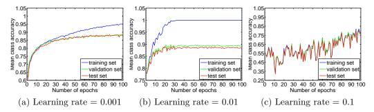
Figure 4: Demonstration of the impact of learning rate. It shows that an over-small learning rate, e.g., 0.001, slows down the learning process, whereas an over-large learning rate, e.g., 0.1, destabilizes the learning process and degrades the classification performance. A better classification result can be obtained by properly tuning the learning rate, as shown in (b).
