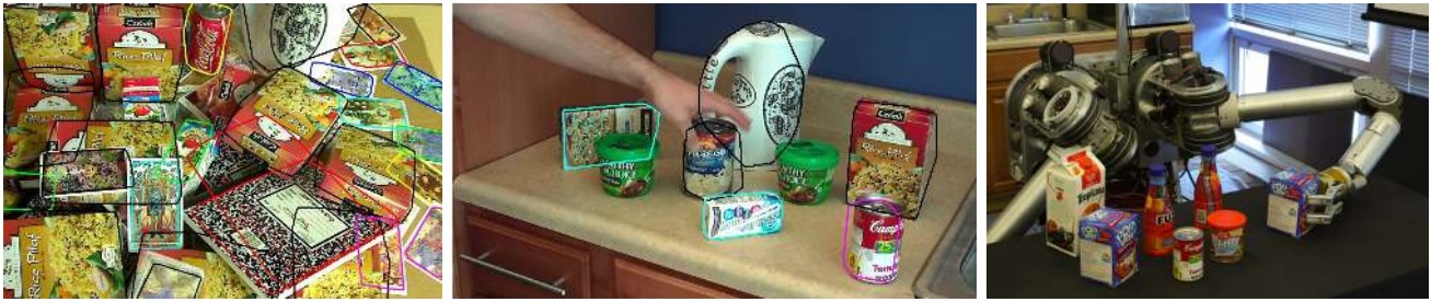
Fig. 9. Recognition of real-world scenes. (Left) High-complexity scene. MOPED finds 27 objects, including partially-occluded, repeated and non-planar objects. Using a database of 91 models and an image resolution of 1600 \times 1200 , MOPED processes this image in 2.1 seconds. (Middle) Medium complexity scene. MOPED processes this 640 \times 360 image in 87 ms and finds all known objects (The undetected green soup can is not in the database). (Right) HERB 2.0 grasping object recognized and registered by MOPED. Images taken from [64].
