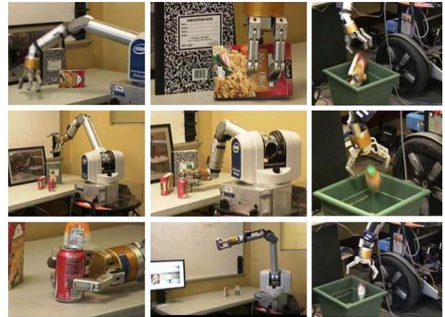
Fig. 13 Snapshots from three runs of the planner on the WAM arm. Top Row: Grasping and throwing away a box of rice. Middle Row: Grasping and throwing away a juice bottle. Bottom Row: Grasping and throwing away a soda can
