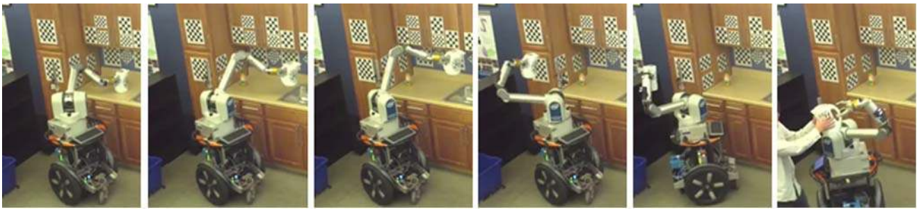
Fig. 12 Snapshots from HERB executing a trajectory for lifting a pitcher ( left to right ). The pitcher is constrained to not tip forward or to the side. This constrained trajectory took less than 5 seconds to plan
