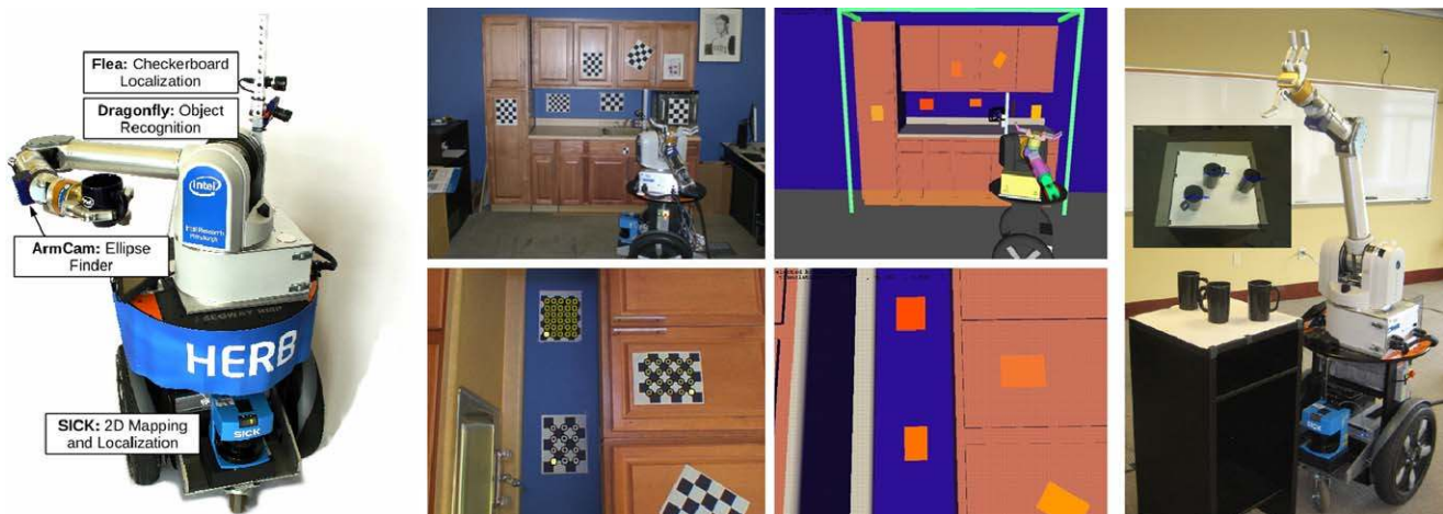
Fig. 3 (Left) Sensors on HERB and the modules that use them. (Middle) HERB uses automatically generated map of checkerboards for refining its localization. Entire scene is shown at the top, and the camera
