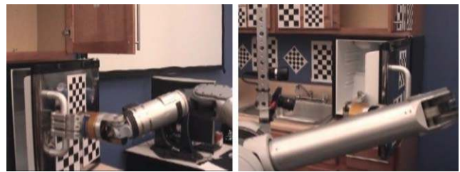
Fig. 11 Herb autonomously opening the refrigerator door by first pulling on the handle and then pushing the door from the inside
