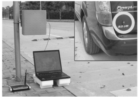
Fig. 10. A local node with a RFID reader and a wireless AP; the highlight area in the inset shows an active RFID tag attached to a vehicle.
