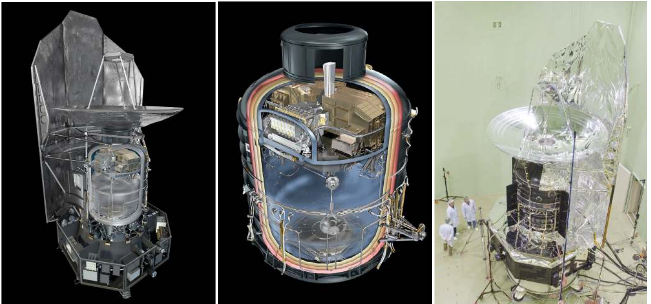
Fig. 1. Left: the Herschel spacecraft features the “payload module” (PLM) with the cryostat housing the instrument focal plane units (FPUs), the telescope, the “service module” (SVM) with “warm” electronics, and the sunshield/sunshade. Middle: close-up of the PLM displaying the optical bench with the instrument FPUs on top of the main helium tank. The focal plane cover and the three vapour-cooled shields inside the cryostat vacuum vessel (CVV) are also shown. Right: Herschel being prepared for acoustic testing in the Large European Acoustic Facility (LEAF) in the ESTEC Test Centre in June 2008, providing a good view of the telescope (ESA).
