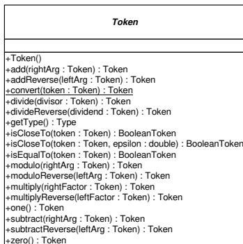
FIGURE 4.2. The Token class defines a polymorphic interface that includes basic arithmetic operations.
