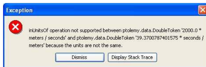
FIGURE 3.11. Example of an exception resulting from a units mismatch.
