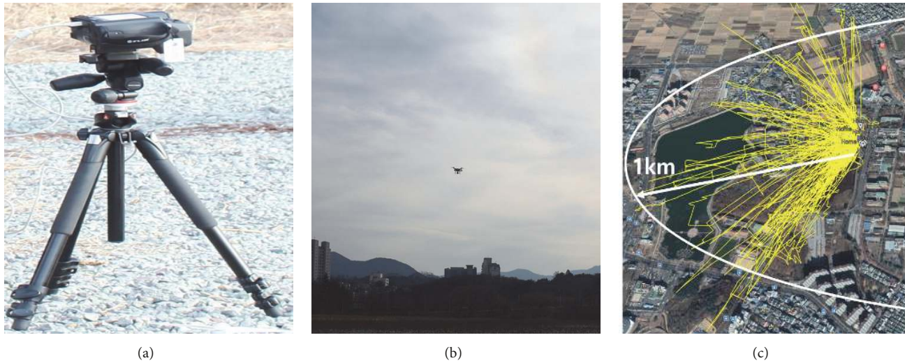
FIGURE 3: Equipment used in the experiment and experimental environment. (a) is a FLIR T620 infrared camera, (b) is a PHANTOM 4 PRO drone model used as a target, and (c) is the flight trajectory of a target.
