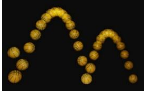
Figure 4. A bouncing ball captured with a stroboscopic flash at 25 images per second. Its trace shapes a parabola. (Source of image: Physics Central.com)
