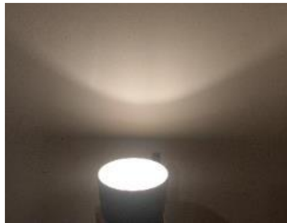
Figure 6. Light spreading shape on a wall forms a parabola (Source of image: authors)
