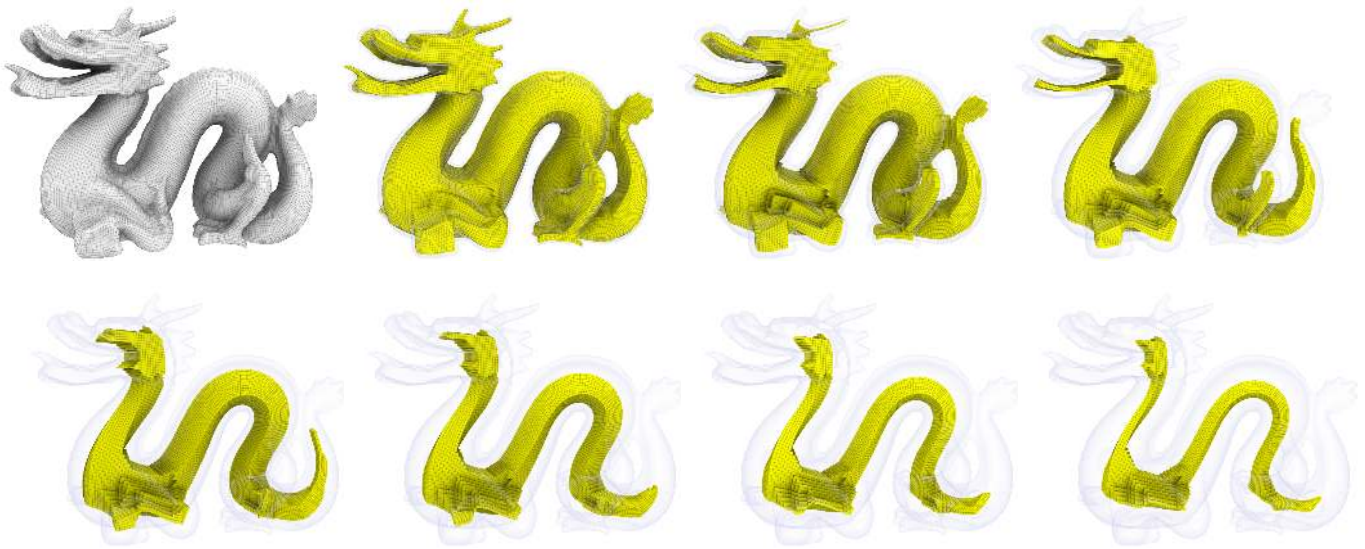
Figure 6: Several layers of peeling reveal hexahedral structure of the dragon follows the overall shape of the dragon. Model courtesy of [18].
