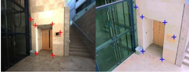
Fig. 4. Left: keyframe obtained when building a map of the scene. Right: view from a surveillance camera. Large changes of viewpoint and illumination make it difficult to automatically find the dominant plane viewed by the SLAM camera and the surveillance camera. It is however a simple task for a user and only needs to be done once. In this image, points have been selected between the two views and provide the input to compute the planar homography {}^o\mathbf{H}_s , linking a plane in the surveillance camera view to the same observed plane in a keyframe belonging to the SLAM map.
