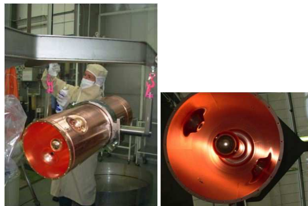
(a) the cavity during the cleaning process (b) internal view of the cavity
