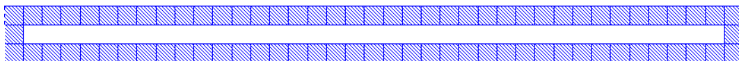
Figure 4.4: Layout of a 78 mm long double folded slot cell with 2 \times 2 mm cell size drawn in Virtuoso. Port label is assigned at the center of the length on the lower slot.
