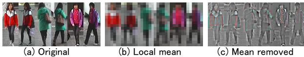
Figure 2. Importance of mean: (a) Original images. (b) Images that show mean RGB values of 10 \times 10 pixel patches of (a). (c) Mean removed images (each RGB value is scaled over the range [0,255] for visualization). It is easy to determine the same persons from (b), whereas it is hard from (c).
