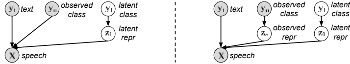
Figure 1: Graphical model representation of the proposed models. Observed class often corresponds to the speaker label. The left illustrates equation 1, and the right illustrates the extension from Section 2.3. The grey and white nodes correspond to observed and latent variables.
