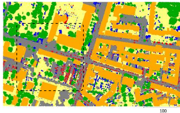
Figure 3. Result of the last CRF^P classification for the test area. The colors correspond to the classes road (grey), natural soil (yellow), low vegetation (blue), tree (green), building (orange), and car (red). The dashed rectangle illustrates the location of Fig. 4
