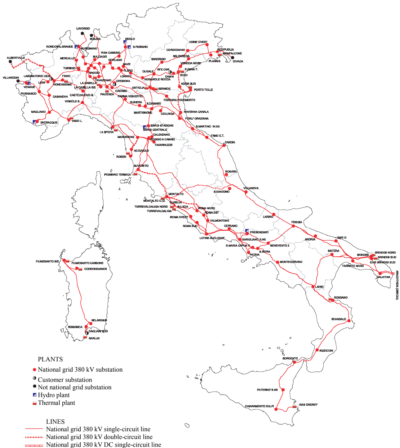
Figure 1. The 380 kV Italian power transmission network.
