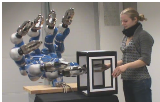
Fig. 1. KUKA LWR 4 robotic arm reaching through a hollow box with task being defined in combined Writhe and interaction mesh space, showing an example of planning and dynamic remapping using topological representations as described in Section V-B.
