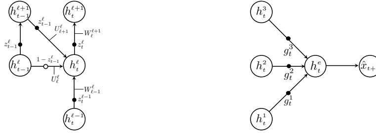
Figure 2: Left: The gating mechanism of the HM-RNN. Right: The output module when L = 3 .
