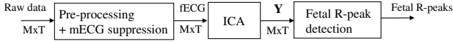
Fig. 1. Block diagram of fetal heart rate detection. M is the number of channels and T is the total time of the recording.
