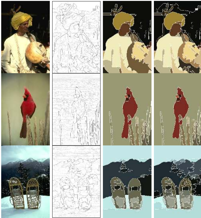
Fig. 10: Hierarchical segmentation results on the BSDS500. From left to right: Image, inverted saliency map, and segmentations at the optimal dataset scale (ODS) and optimal image scale (OIS).
