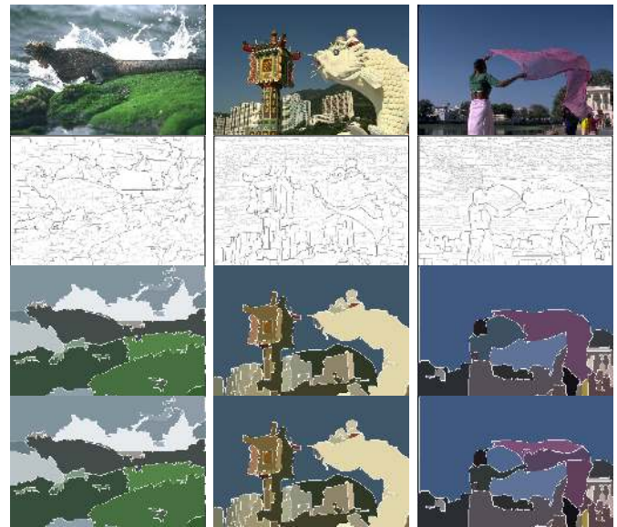
Fig. 11: Additional hierarchical segmentation results on the BSDS500. From top to bottom: Image, inverted saliency map, and segmentations at the optimal dataset scale (ODS) and optimal image scale (OIS).
