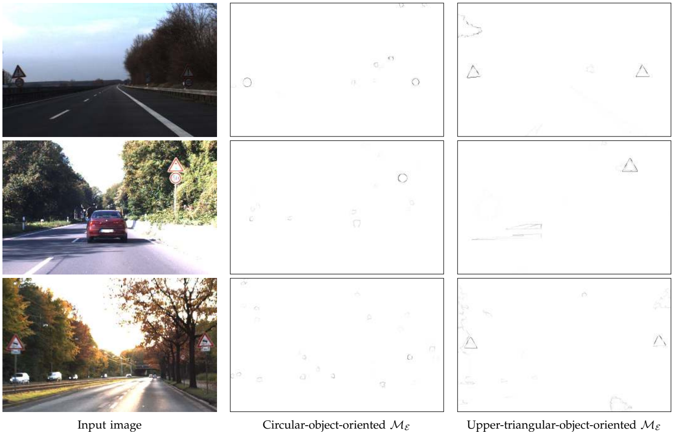
Fig. 13: Qualitative illustrations of shape-oriented saliency maps on some images from GTSDb test dataset [40].
