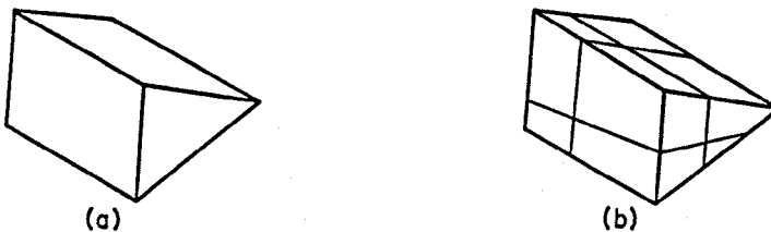
Figure 11. (a) Example three-dimensional object; and (b) its corresponding PM_1 octree.
