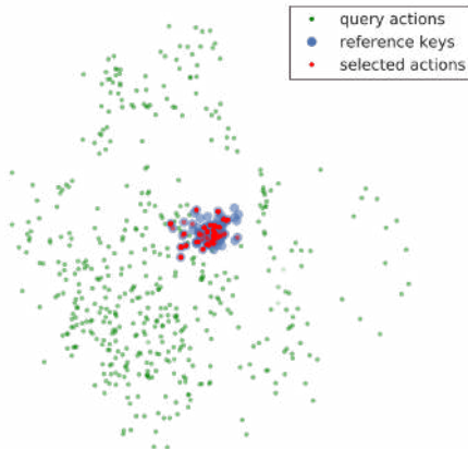
Figure A.3: Visualization (using PCA) of the actions produced by the trained query-based policy (on go-to-target). Query actions are the continuous actions generated by the policy. Reference keys are the feature vectors associated with the control fragments (here, features of the final state of the nominal trajectory of the fragment). Selected actions are the actions produced by the sampling mechanism and they are overlain to emphasize the control reference keys actually selected. The most prominent feature of this visualization is the lack of precision in the query actions. Note that 45/105 control fragments were selected by the trained policy.
