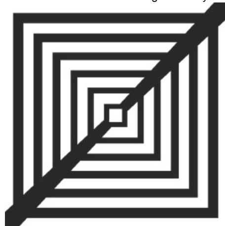
Figure 27. Parallel channel flow field design incorporating Murray's branching law design. [142a] Copyright© 2010 Wiley.
