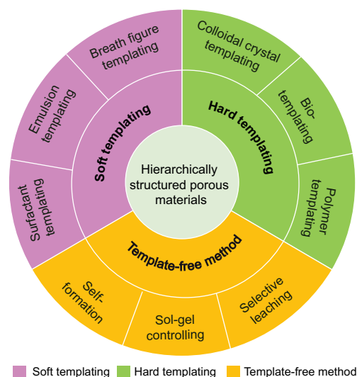
Figure 1. Illustration of various technologies for the synthesis of hierarchically structured porous materials: soft templating (surfactant templating, emulsion templating and breath figure templating), hard templating (colloidal crystal templating, bio-templating and polymer templating), and template-free method (self-formation, sol-gel controlling and selective leaching).
