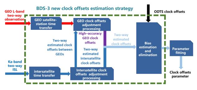
Figure 4. The procedure of the BDS-3 new clock offsets estimation strategy.
