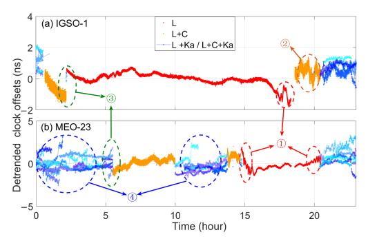
**Figure 3.** The typical one-day detrended two-way clock offsets of IGSO and MEO measured by BDS-3 two-way superimposition strategy. ①–④ describe the problems and abnormal phenomena in the two-way superimposition strategy.
