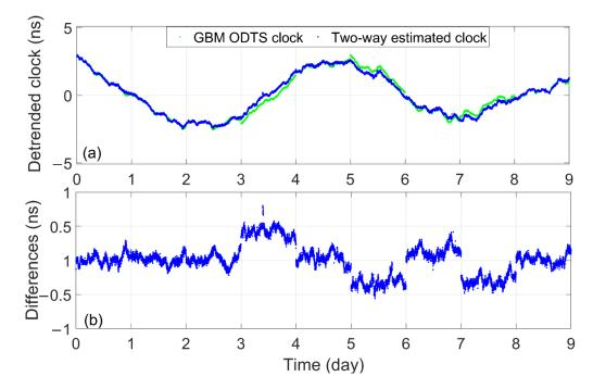
**Figure 10.** 9-day Satellite clock offset differences between the Ka-band inter-satellite estimated clock offsets and GBM products. Wherein, (a) describes the two kinds of clock offsets after deducting the same trend. (b) describes their differences. The reason why "hop" exist in the bottom figure is that the day-boundary discontinuities exist in the ODTS clock offsets (since 19 May 2022).
