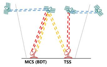
**Figure 1.** The construction of BDS time synchronization and the basic two-way measurements of BDS-3. Wherein, the red, blue, yellow curves are L-band satellite-station two-way measurements, Ka-band inter-statellite measurements, C-band inter-station two-way measurements, respectively.
