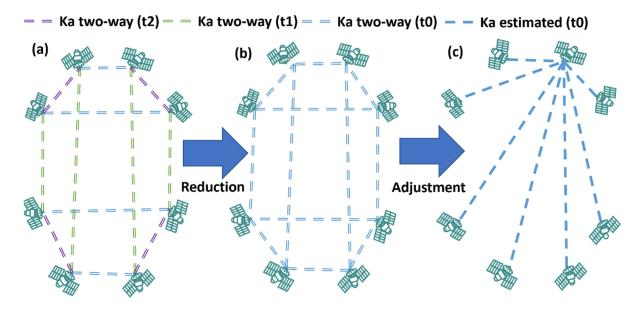
redundant Ka-band inter-satellite two-way clock can be used to estimate the clock offsets with higher accuracy (see Figure 5c) [19].
