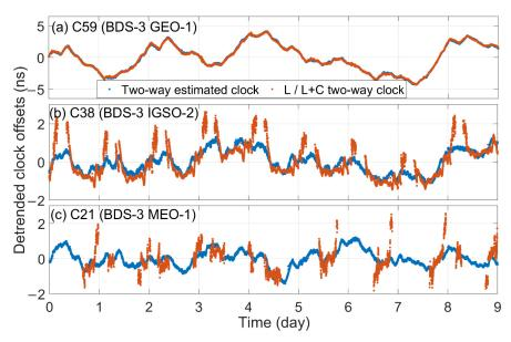
**Figure 12.** Satellite clock offset differences between the two-way estimated clock offsets and the two-way intraregional satellite clock offsets measured by superimposition strategy (since 19 May 2022).
