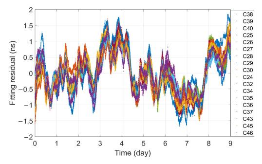
**Figure 13.** Multi-day fitting residuals of BDS-3 satellite with highest-level-performance atomic clock onboard with respect to BDT (since 19 May 2022). The common fluctuation is caused by the fluctuation in BDT output signals.
