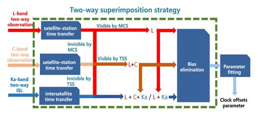
Figure 2. The procedure of the BDS-3 two-way superimposition strategy.
