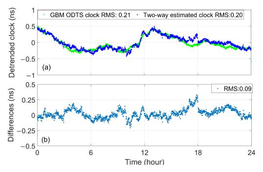
**Figure 9.** 1-day Satellite clock offset differences between the Ka-band inter-satellite estimated clock offsets and GBM products (since 19 May 2022). Wherein, (**a**) describes the two kinds of clock offsets after deducting the same trend. (**b**) describes their differences.
