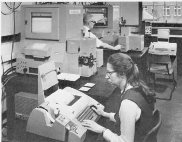
PLATE 4. View of the NPL on-line spectrophotometry data-system, showing the Cary 14 and 14R instruments. The near one is fitted with the Cary 1411 small sphere attachment, and the far one is fitted with the large sample compartment with box-lid extension for transmittance work on long samples.
